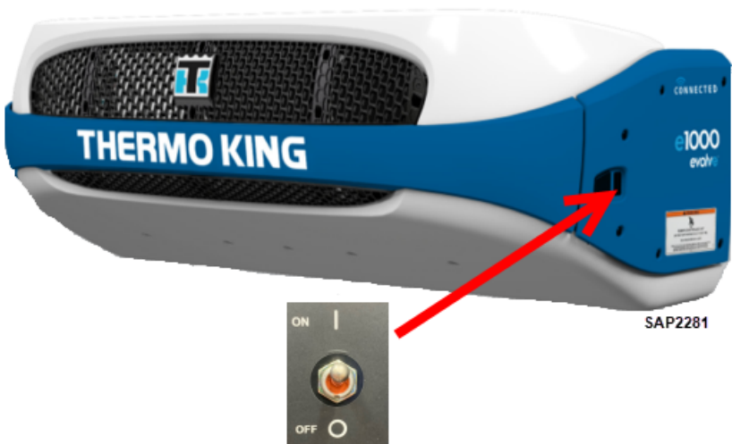
Figure 9. Unit Service Switch location shown
